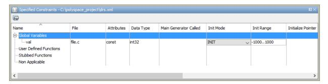
To see the Specified Constraints window, with the Bug Finder results open, select **Window > Show/Hide View > Specified Constraints**.
